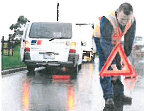
Low risk example. Prominent warning signs for approaching drivers.
