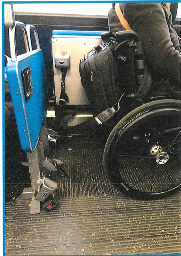
Figure 2. Incorrect tiedown in use, photographed by the researchers in USA, 2018.
