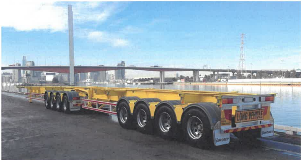
Figure 10 – A B-Double combination with two quad axle groups (source: supplied by Vawdrey Australia)
