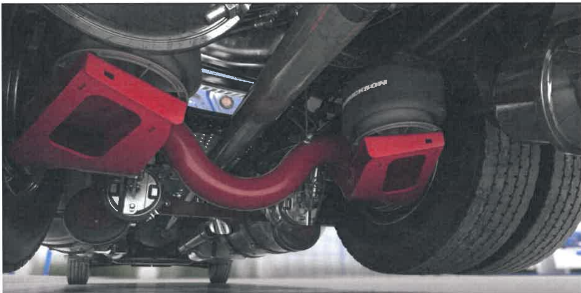
Figure 7 – Underbody view of a truck with a leading retractable axle (note the bend in the red axle around the driveshaft) (source: supplied by Hendrickson Asia Pacific)
