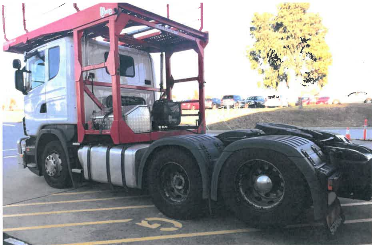
Figure 9 – A prime mover with a trailing retractable axle (source: supplied by Scania Australia)
