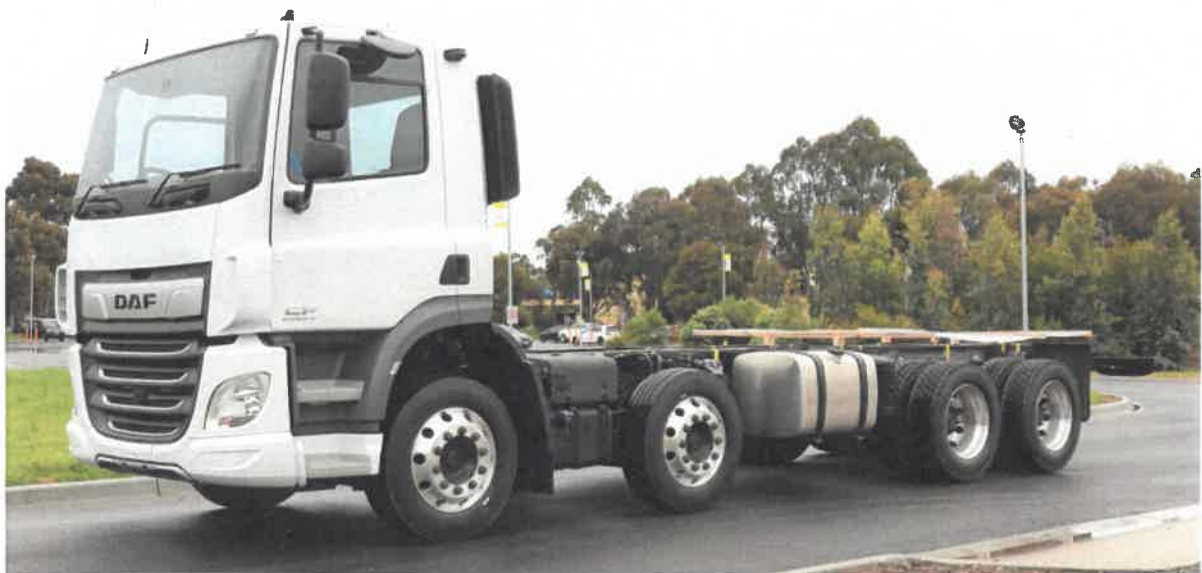
Figure 5 – A heavy rigid truck (cab-chassis) with a twin steer axle group (source: supplied by Paccar Australia)
