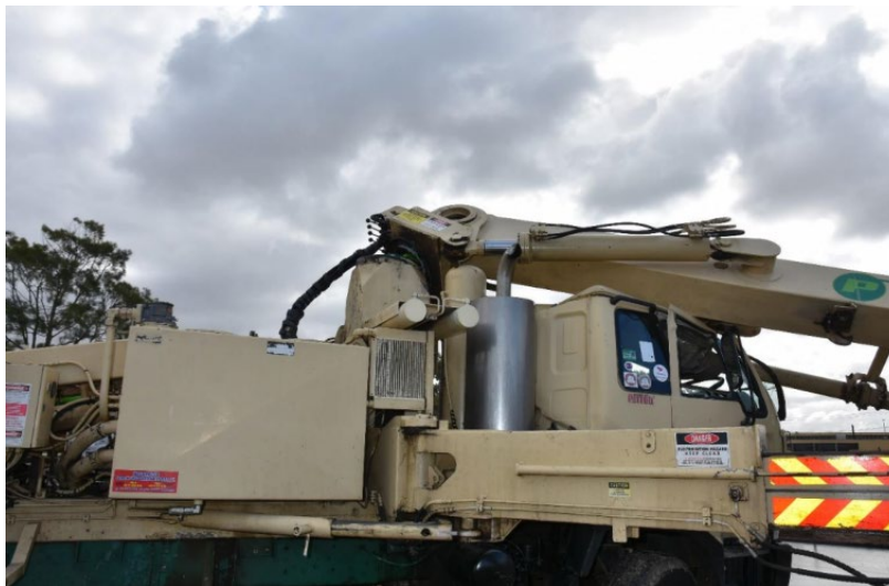
Photo of the snapped king post taken following its collapse.
